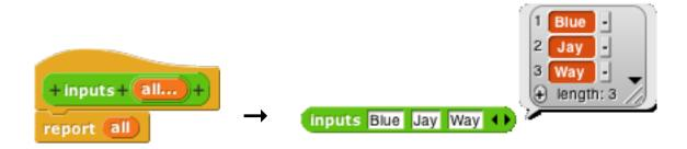
The ellipsis (...) in the orange input slot name box in the prototype indicates a Multiple input.
